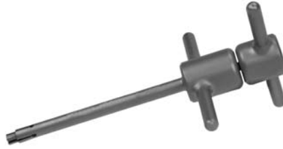
Fig 25. Detail of attaching the new hinge pin to the extractor
